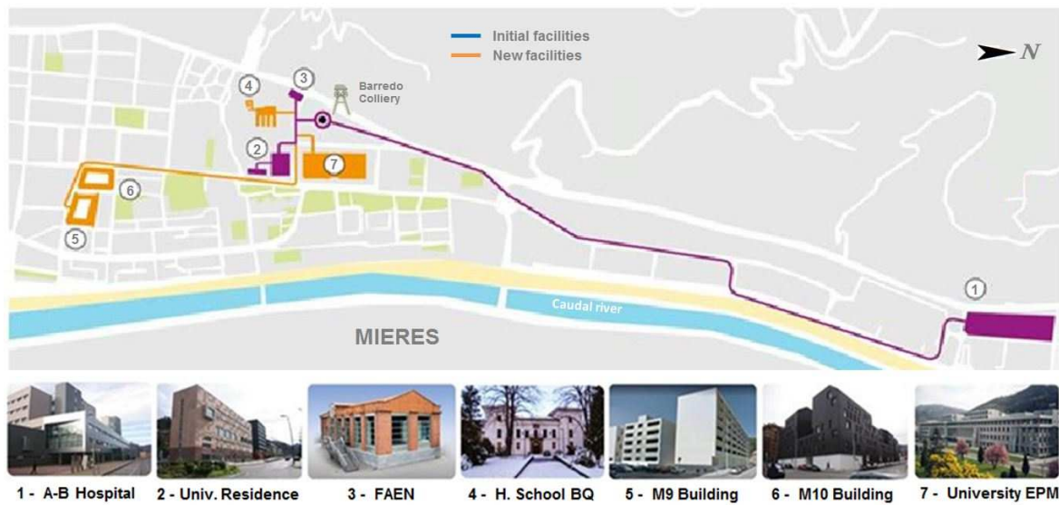
Scheme of District Heating in Barredo Colliery
