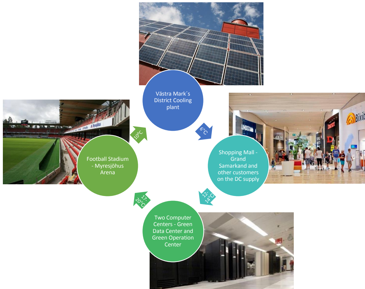
Figure 5. Innovative district cooling cycle network in Växjö
