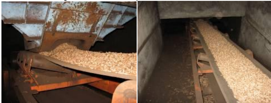
Fig. 3 Conveyor with pellets.
