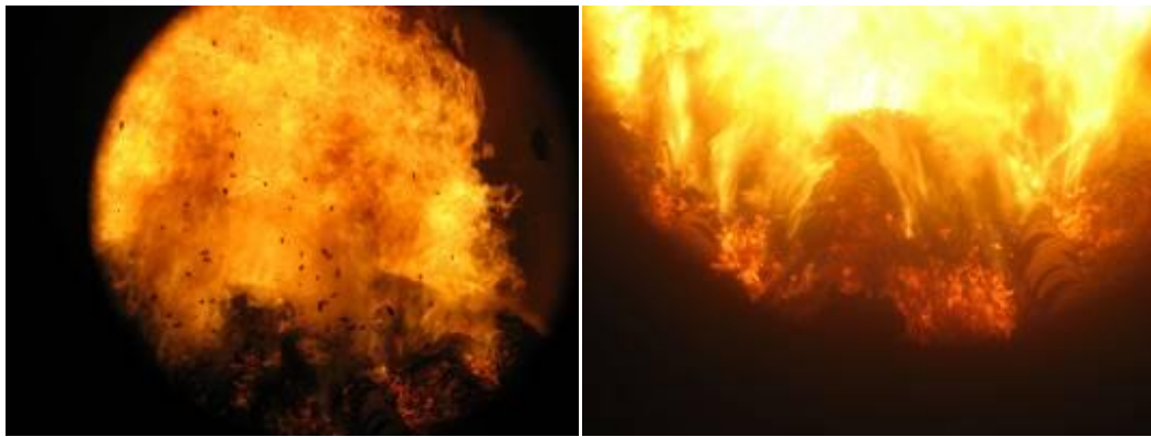
Fig. 5 Combustion of pellets. View from the inspection window.
