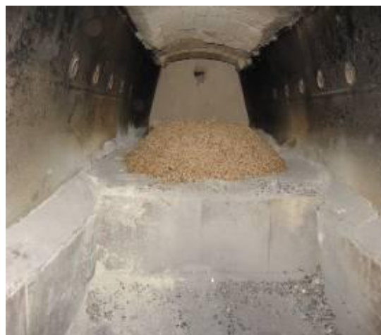
Fig. 1 Pellets in furnace during fuel consumption rate measurements
