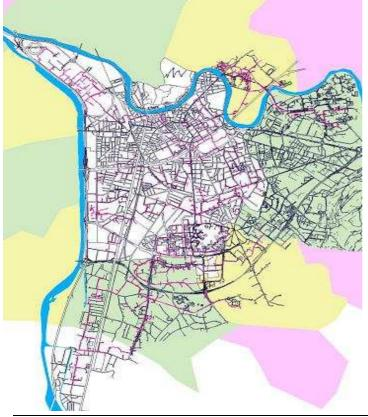
Supplied with superheated water by six totally interconnected heating plants, the network supplies more than 900 public or private buildings all along the 160 km of underground heating ditches. A Digital Control System (DCS) enables heating requirements to be anticipated and the power to be adjusted at all times giving priority to the most suitable fuels.
