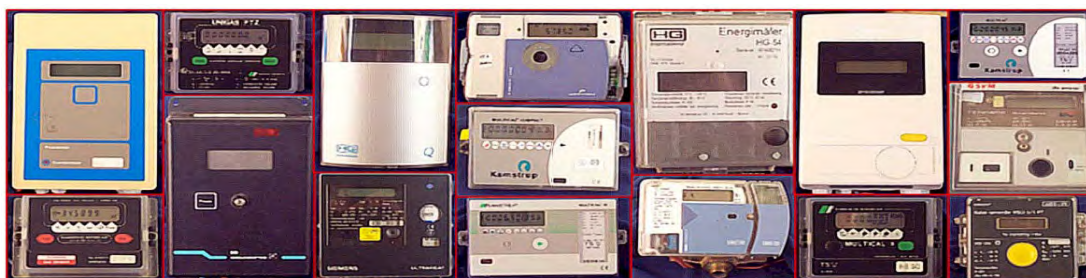
Illustration 20: Different types of meters used in DH installations through the years.
