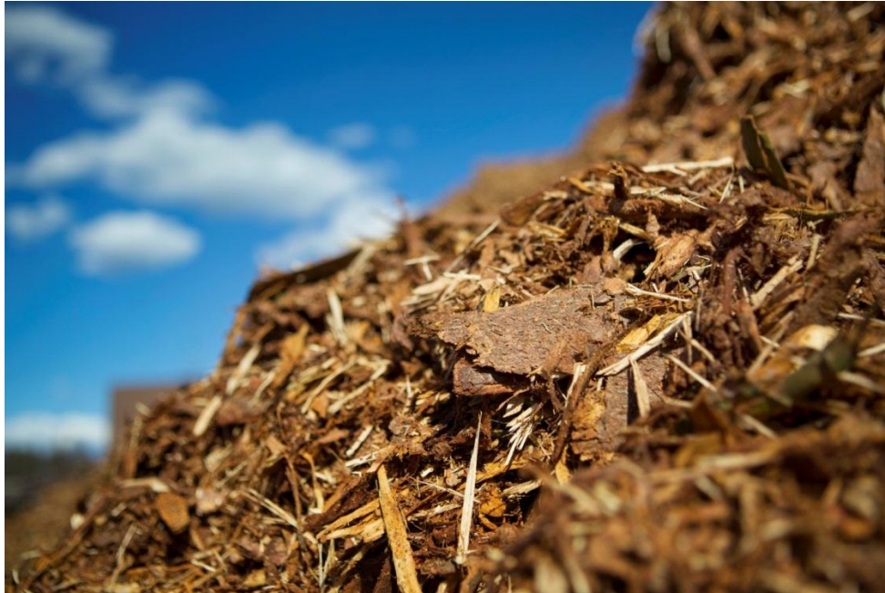
Picture 1. Typical biofuel of CHP plant in Joensuu.
