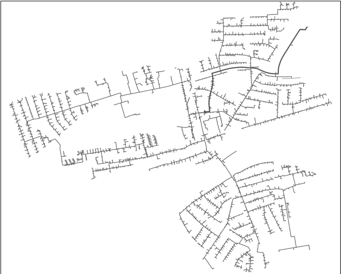
Fig. 3.1 The configuration of the DH network in Bjerringbro. The thin lines show the distribution network, which is directly connected to the consumers. The thick lines show the transmission line connecting the CHP-plant, Energicentralen and the boiler station.
